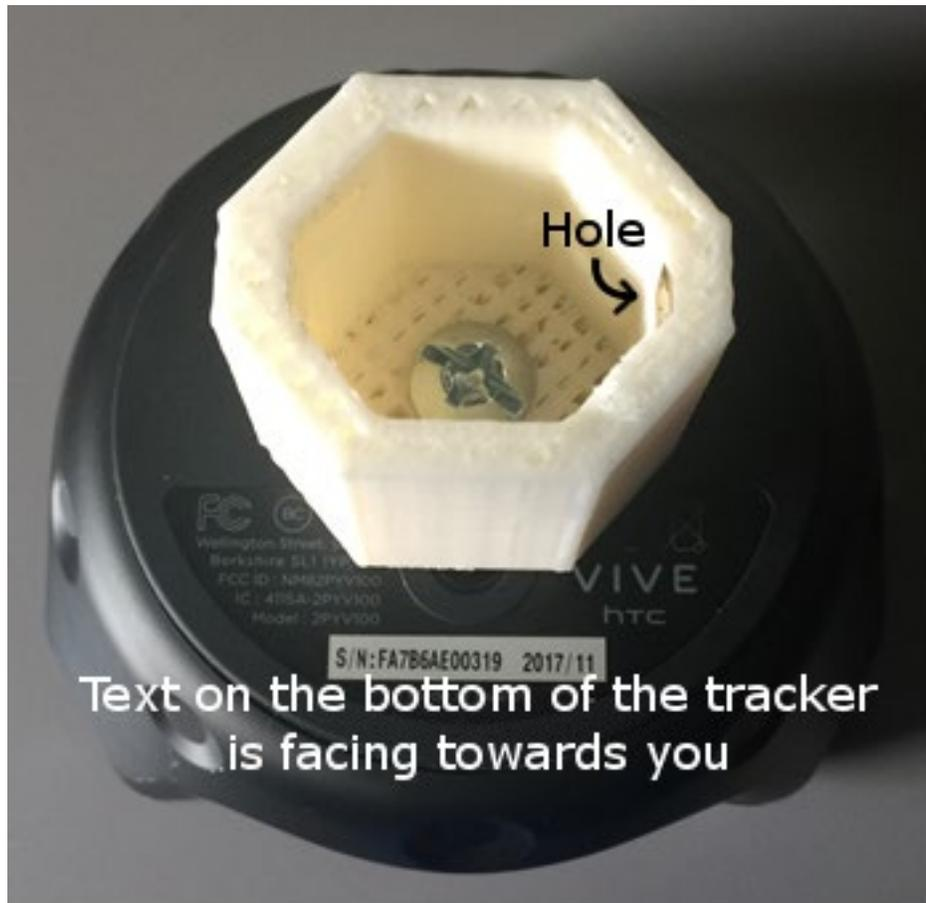
**The hole in the mount is facing to the right when the text on the bottom is facing towards you**
